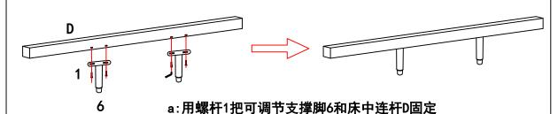
a: Use the Big Screw(1) to secure the Adjustable support feet (6) to the Middle Slat[D].
